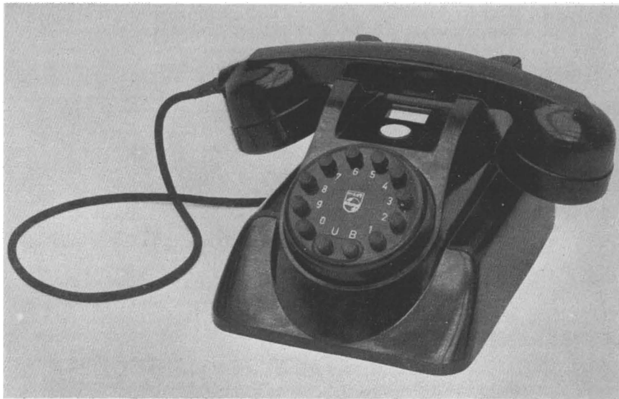
Fig. 7. Keysending telephone set.
